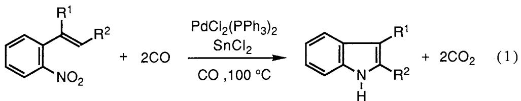
In a typical experiment, a mixture of *o*-nitrostyrene derivative (2.0 mmol),  $\text{PdCl}_2(\text{PPh}_3)_2$  (0.10 mmol), and  $\text{SnCl}_2$  (1.0 mmol) in 1,4-dioxane (10 ml) was stirred at 100 °C for 16 h under carbon monoxide pressure (20 kg/cm<sup>2</sup>). All products were isolated by Kugelrohr distillation, and satisfactory spectroscopic and analytical data of them were obtained.
